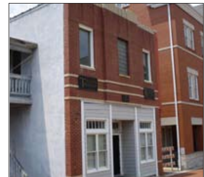
Adjacent 2 and 3-story facades in Dallas. Note that the taller building actually has a 4th floor, but the facade is only 3 stories and is in scale with adjacent buildings.
